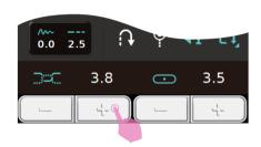
Press the "+" or "-" button to adjust the stitch tension.
