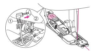
Attach the electronic buttonhole foot and plug the cord into the socket behind the face cover.
