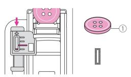
The buttonhole length may need to be decreased for thin button, adjust the pointer toward to "-" for fine tuning.
