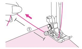
2. Place the fabric under the presser foot, pass the thread under the presser foot, and then pull out about 10cm of thread toward the rear of the machine.
