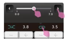
Click the Needle position icon and a slider will pop out for quick value adjustment. Click anywhere on the screen to leave the window. Click the Needle position value icon will reset the value to default.
