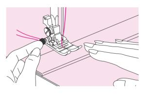
When you reach the point of an increased thickness, lower the needle and raise the presser foot lifter. Press the toe of the foot to the horizontal line and push in the black button, then lower the foot and continue sewing.
