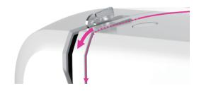
Continue to guide the thread into the silver discs to keep the thread in proper tension.
