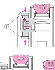
Consider the shape and height of each button, buttonhole fine tuning adjuster provides fine adjustment of the buttonhole length.
