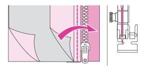
Turn the fabric right side out. Attach the left pin for sewing the rightside of the zipper.
