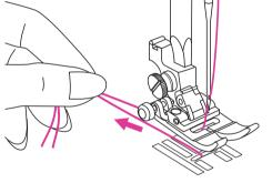
Pull both threads to the back under the presser foot.
