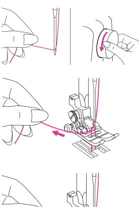
Hold the upper thread with your left hand. Turn the handwheel towards you (counterclockwise) to lower the needle down below the needle plate then raise it to bring the bobbin thread up.
