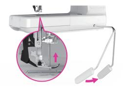
Push the knee lifter with the knee to the right to raise the presser foot. Simultaneously the thread tension is released.
