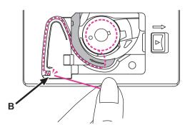
To cut off excessive thread, pull it to the cutter at point (B).
