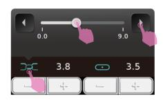
Click the Thread tension icon and a slider will pop out for quick value adjustment. Click anywhere on the screen to leave the window. Click the Thread tension value icon will reset the value to default.
