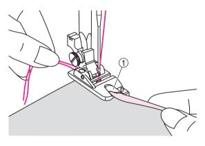
Insert the needle into the fold by turning the handwheel toward you, and lower the presser foot lifter. Sew several stitches and raise the presser foot lifter.
