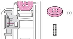
The red mark is the standard setting for regular button, adjust the pointer align with the red mark.
