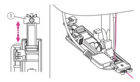
Extend the button holder plate and set to the desire length. Adjust the stitch width and the stitch length to the desired width and density.
