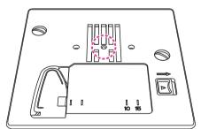
Change the straight stitch plate and tighten the screws.
