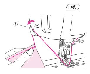
6. Press the thread cutter button to trim the threads.
