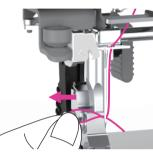
12. Raise the lever, the hook will rotate and pass the thread through the needle eye to form a loop.
