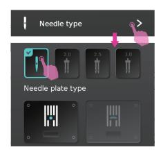
After changing to straight stitch plate, please go to needle type setting and choose single needle, the machine will automatically sensor which needle plate is using.
