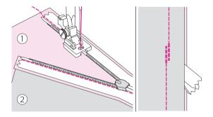
To attach the other half of the zipper, pin tape face-down with coil on seam line (1.6cm) and top stop 1.9cm below raw edge of garment, as before. Make sure that the zipper is not twisted at the bottom. Use the left-hand groove of foot, making sure that the center marking is still lined up with the needle and stitch, as before.
