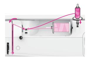
Set the second spool pin into the hole on the top of the machine and put spool pin felt and thread onto second spool holder.
