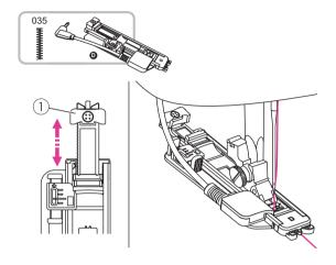
Using the electronic buttonhole foot.
