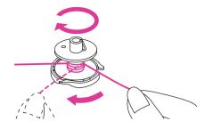
5. Wind the thread clockwise around the bobbin 5-6 rounds.
