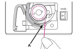
Pull the thread through the slit (A).
