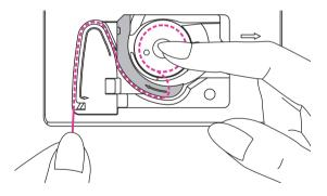
With a finger hold gently on top of the bobbin, please follow the arrow markings and draw the thread into the bobbin thread guide.
