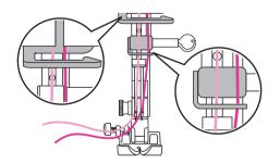
As shown in the picture, pull the thread from the horizontal spool holder pass through left needle hole manually and thread from the second spool holder pass through right needle hole.
