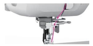
8. Pass the thread behind the flat, horizontal thread guide. Threading to the right side of the thread guide.
