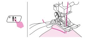
3. Press the needle up/down position button to lower the needle into the fabric at the beginning of the stitching.
