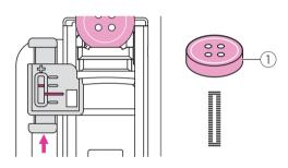
The buttonhole length may need to be increased for thick button, adjust the pointer toward to "+" for fine tuning.
