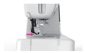
Swing the DFS mechanism forward under the back of the presser foot until it is engaged and stays in the lowered position.
