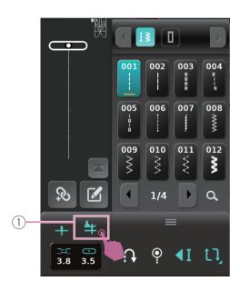
When you want to change the sewing direction, you can also set the pivot function in the sewing mode. When you stop sewing, the needle will stay in the fabric, and presser foot will automatically lift, which can easily rotate the fabric. This function is very useful. (Presser foot height setting, please refer to "setting" chapter for more information.)
