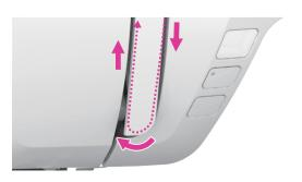
Pass the thread under the take-up spring then pull it upwards as arrow marks illustrated.
