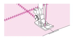
Working on the right side of the fabric, place the center of the presser foot on the seam line of the joined fabrics and stitch over the seam.
