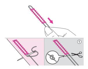
Once sewing is completed, pull the gimp thread gently to remove any slack. Cross the gimp in front of the needle and thread gimp ends into a large needle, pull to the wrong side and knot ends before cutting excess.
