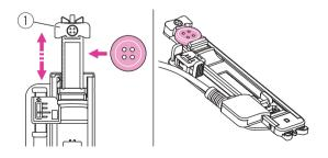
Pull the button holder plate to the back, and place the button in it. Push back the button holder plate against the button to hold it tight.
