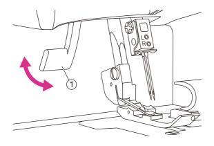
Raise the presser foot with the presser foot lifter at the back of the machine.
