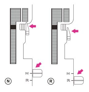
The stitch finger lever should be set to "N" (Normal) for all standard overlock sewing. To sew rolled edge you need to retract the stitch finger by setting the stitch finger lever to "R" (Rolled Edge). When moving the stitch finger, be sure to push the lever as far as it will go in each direction.
