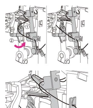
Hold the thread end with your left hand. Use the tweezers to place the thread behind the fingers of the lower looper threader.
