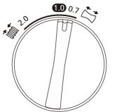
The differential feed system consists of two sets of feed teeth arranged one behind the other. Both feed teeth work independently of each other to provide good results when sewing on speciality fabrics. When the amount of feed by the front feed teeth is changed in relation to the feed by the rear feed teeth it will "stretch" or "gather" the fabric.
