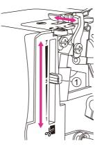
The stitch width can be increased or decreased by changing the needle position or with the cutting width lever.
