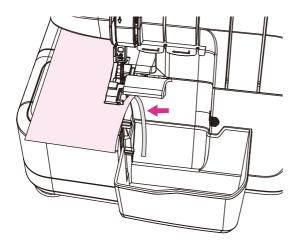
When sewing, the fabric scrap will fall along the front cover into the waste collector.
