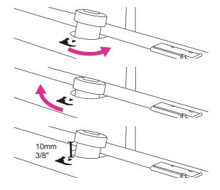
The presser foot pressure is pre-set for sewing on medium weight fabric. When sewing in different fabric weights, adjustment might be needed. Generally, decrease the presser foot pressure when sewing in light weight fabric and increase it when sewing in heavy weight fabrics. Always test sew on a sample of your fabric before sewing on your project. Increase or decrease the pressure in small increments by turning the presser foot pressure screw.
