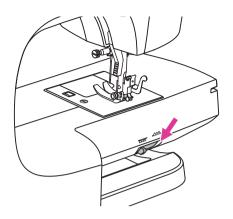
The drop feed lever can be seen on the base at the back side of the sewing machine.
