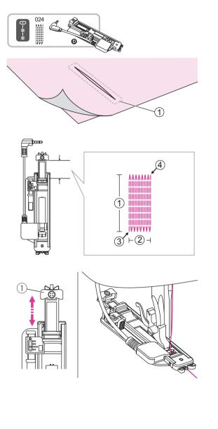
Using the electronic buttonhole foot.
