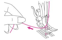
Hold the upper thread with your left hand. Turn the handwheel towards you (counterclockwise) to lower the needle down below the needle plate then raise it to bring the bobbin thread up.
