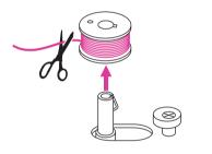
6. Hold the thread tail securely in one hand. Step on the foot control or press the start/ stop button to start winding the bobbin.
