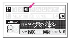
During machine is sewing: When Direct Pattern Group number 6-9 or Regular Pattern Group number 001-008 or 026-099 or Quilting Pattern Group 000-046 or 048-049 is selected, the machine will sew 3 locking stitches at the end of the current stitch if the auto-lock button pressed. Then it will stop automatically. The function can be cancelled if pressed the button once again during sewing.
