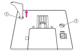
Change to straight stitch needle plate and tighten the screws.
