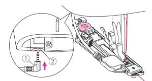
Attach the electronic buttonhole foot and plug the cord into the socket above the presser foot bar.
