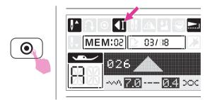
During machine is sewing, the machine will sew 3 locking stitches at the end of the current stitch if the auto-lock button pressed. Then it will stop automatically. The LCD screen will display the auto-lock icon. If pressing the start/stop button again, it will sew from the next stitch.
