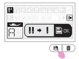
Make sure that the twin needle is not used and it is single needle only. Press the memory button to finish the setting.
