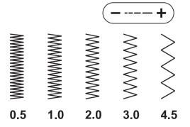
Press the stitch length adjustment button "+" or "-" to adjust the stitch length.
