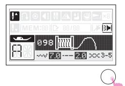
After selecting the pattern, long press the pattern group switch button to enter the stitch balance adjustment mode.
