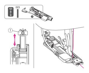
Using the electronic buttonhole foot.
