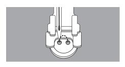
Select the zig-zag stitch and adjust the stitch width according to the distance between the two holes of the button.
