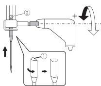
When inserting a new needle, keep the flat side of the shaft to the back.
