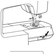
The drop feed lever can be seen on the base at the back side of the sewing machine.
