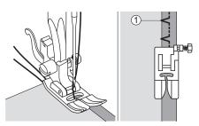
Place the fabric under the foot. Turn the handwheel forwards until the needle swings fully to the left. It should just pierce the fold of the fabric.
