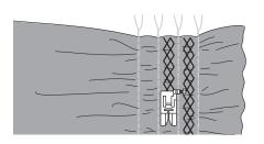
Reduce the tension if necessary and sew decorative stitches between the straight seams.
