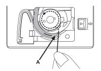
Pull the thread through the slit (A).
