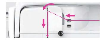
Guide the thread forward and pass through upper thread guide.
